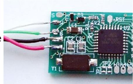
**Warning:** Some rare USB cables dont follow the standard color code. If the cable you use has additional wires, if any color is different, or if you have doubts, check the pinout with a multimeter. Mis-wiring may cause damage to your computer, to this circuit or to the controller.
