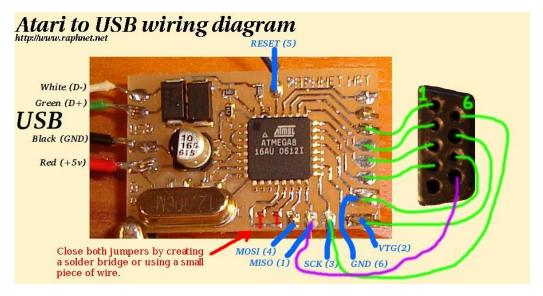
**Note:** The blue wires on the diagram above are for (re)programming the microcontroller. Useful if you want to customize the software.
