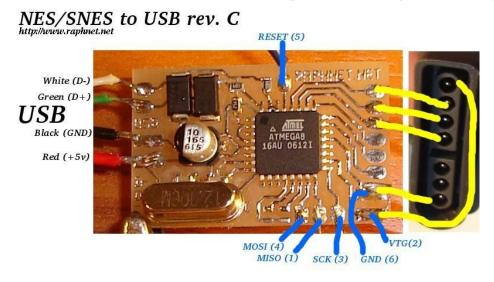
**Note:** The blue wires on the diagram above are for (re)programming the microcontroller. Useful if you want to customize the software.
