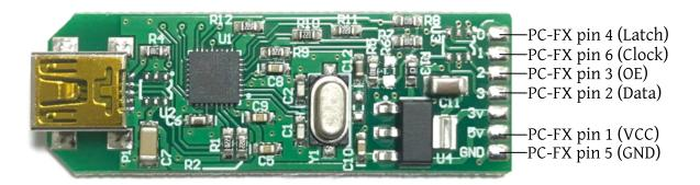
Pin numbering corresponds to what is written on the circuit board inside the controller. If you are cutting a controller cable, or building an adapter from controller ports salvaged from a broken console, use a continuity tested to determine which color goes where.
